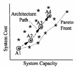
Figure 2 Example of a path in trade space [Source: de Weck et al. 2004]
